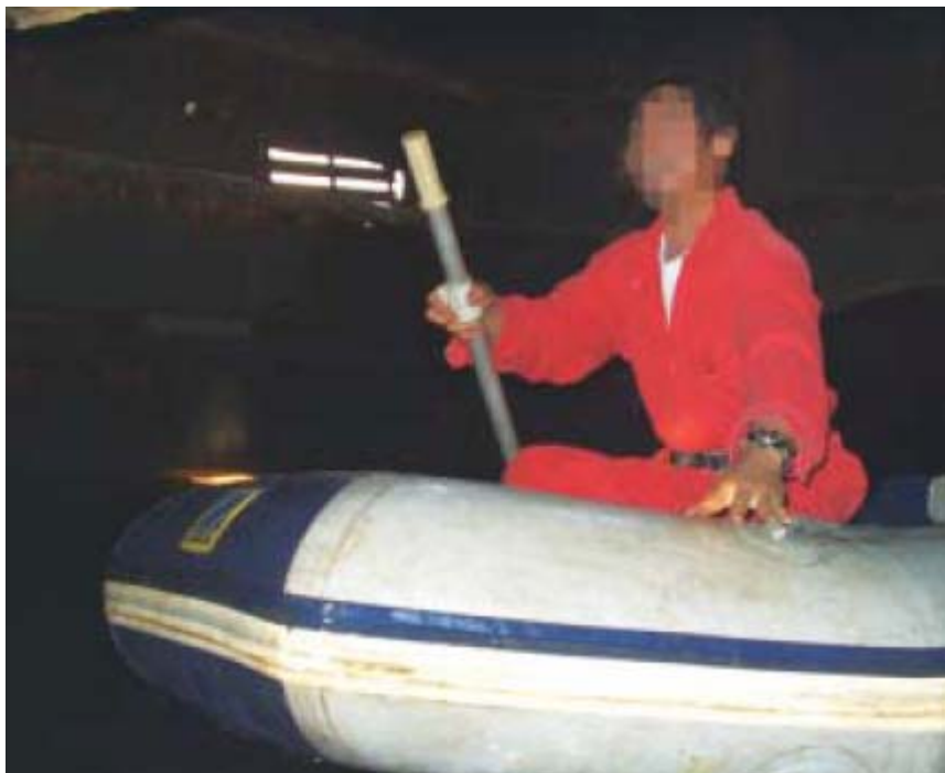
Rafting in cargo tank.
