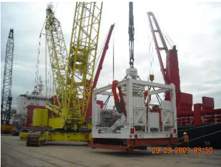
129 mt BOP being loaded by Shore Crane
