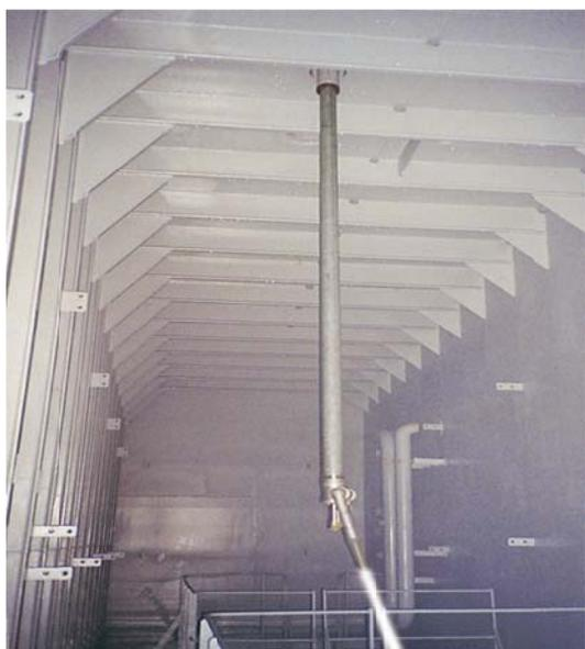
*Tank Cleaning machine in operation.*
