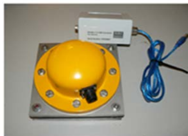
Figure 11: SIRI Marine spatial motion and acceleration sensor
