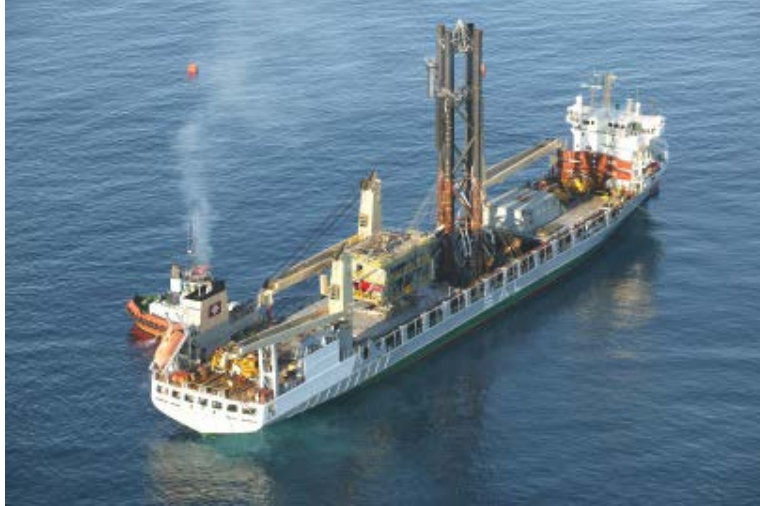
Figure 2: SAL's MV Annegret with jacket top positioned on the double bottom
