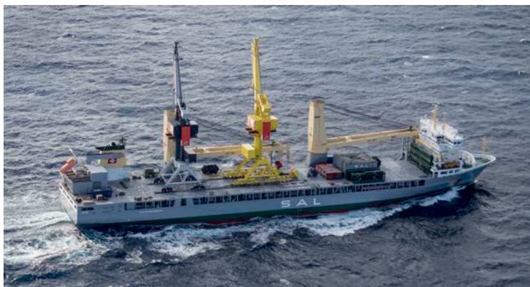
Figure 1: SAL's MV Lone with two port cranes sea-fastened on deck
