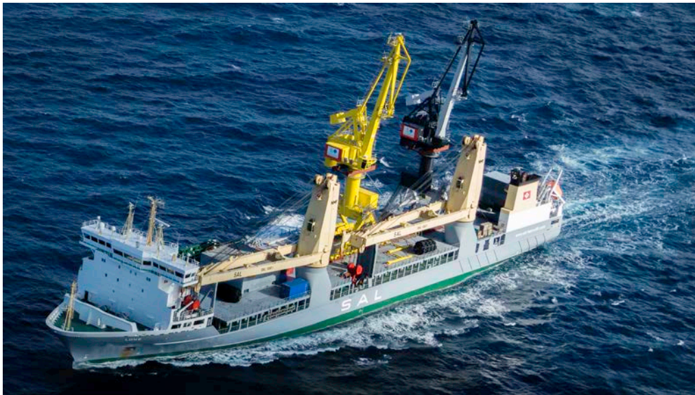
Figure 3: Deck-stowed cranes on SAL's MV Lone
