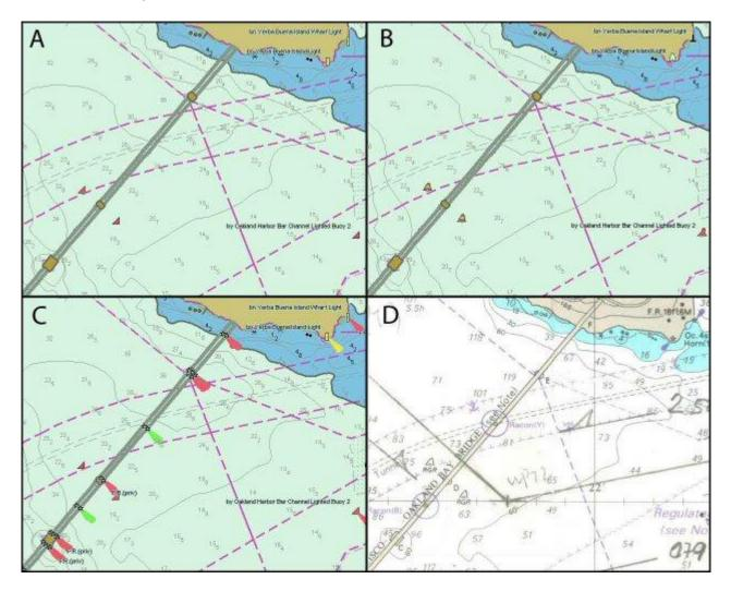
These chartlets display the variations of how this geographical area can be displayed on the ECDIS. Figure A is simplified ENC symbols. Figure B is traditional symbols. Figure C is illuminated ENC symbols and Figure D is the paper chart.
