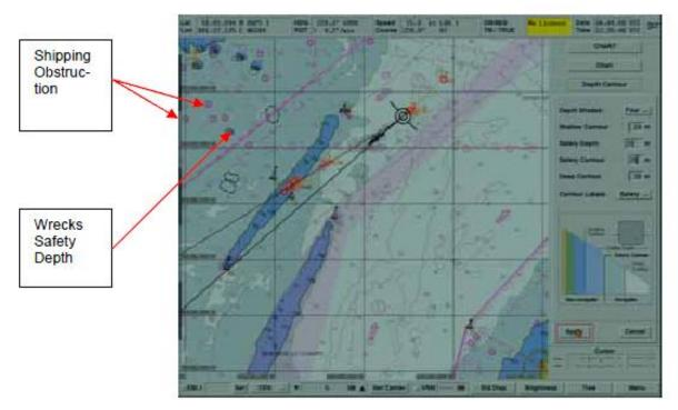
With the safety depth and safety contour set on 20 meters, the display grows even clearer. The passage between both sand banks is visible and more shipping obstruction and less wrecks are displayed.
