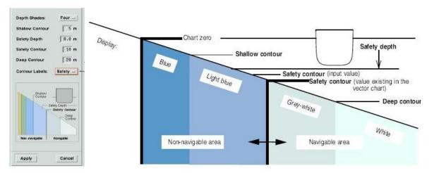
The below image demonstrates how an ECDIS, displays information on a four colour ECDIS.
