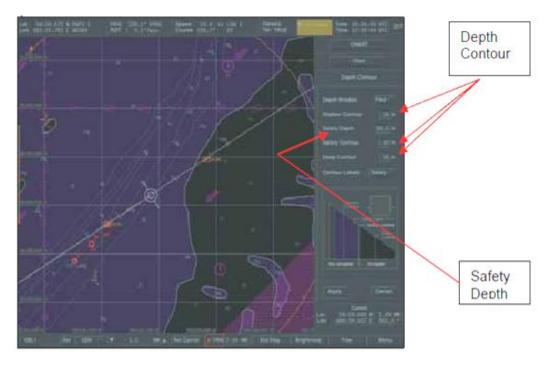
In the picture above the same settings are used as before, 30 meter safety depth, however in this case the ECDIS is set for night mode only showing two colours. The sand bank, as well as the buoy symbols (note symbols are set to traditional not simplified making them almost undetectable), are not prominent as they are already in the unsafe area, where according to the definition, no maritime shipping should take place and therefore should be avoided.
