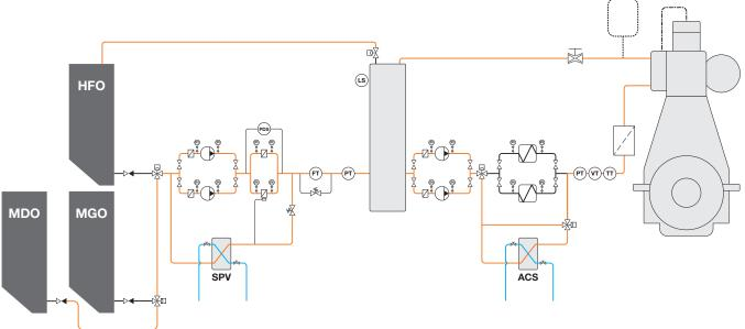
The Alfa Laval Automated Fuel Changeover System (ACS) safeguards the changeover from HFO to gas oil and vice versa. It secures the cooling of the gas oil needed to meet the engine manufacturer's specified viscosity. Everything is done safely and reliably at the push of a button, ensuring peace of mind.
