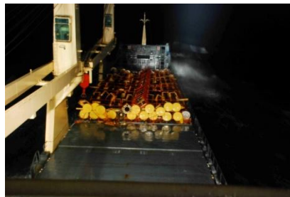
Pipes breaking stow
