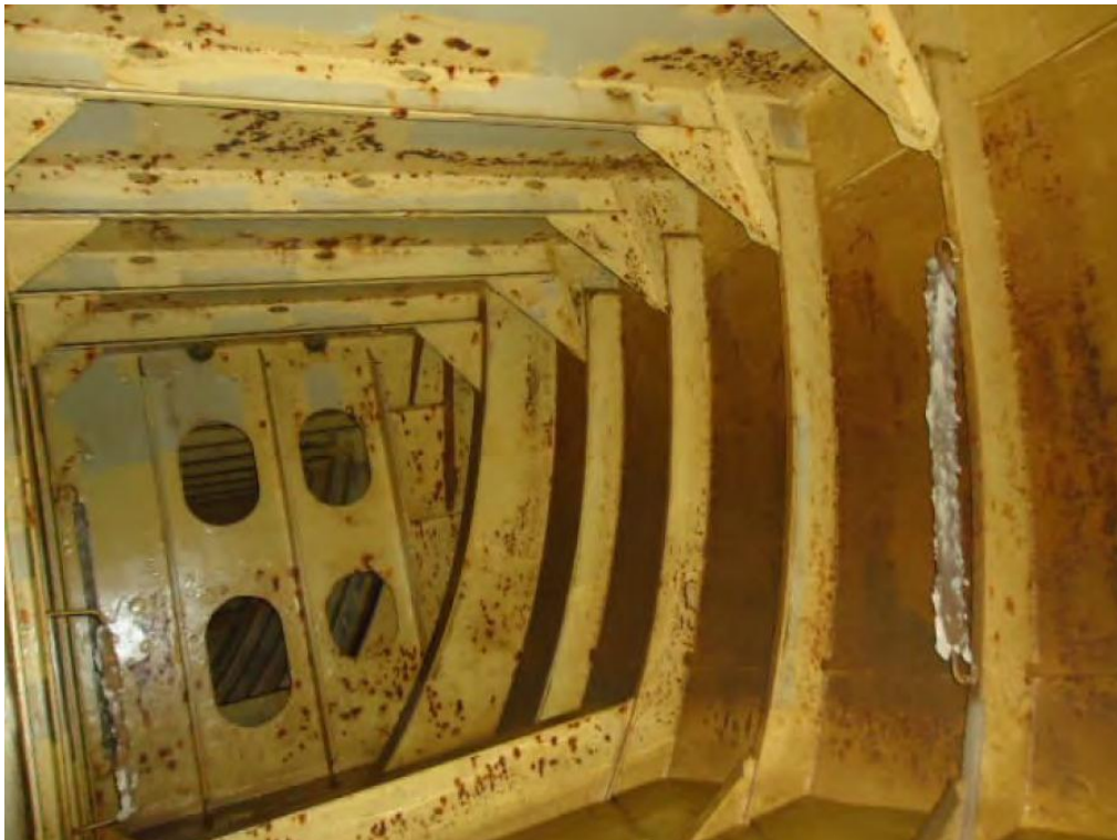
A Water Ballast Tank, empty. When filled it can be the unintended “passenger” compartment for a significant variety of marine life.
