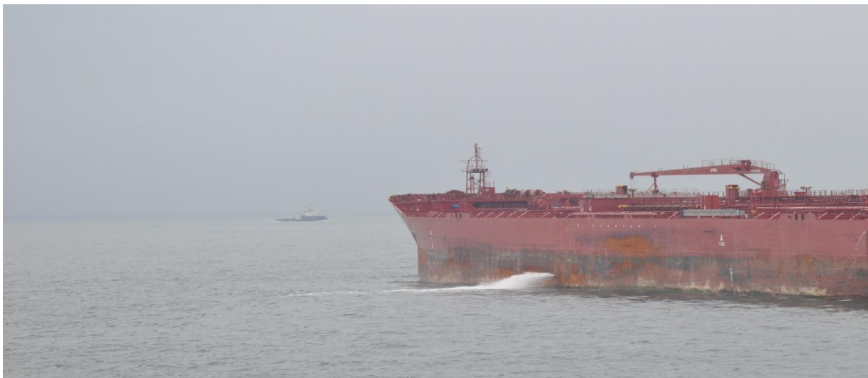
Vessel engaged in pumping out.
