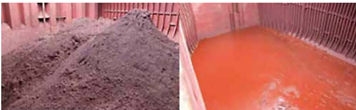
Figure 10 - Iron ore fines before and after liquefaction (Photo: Gard)
