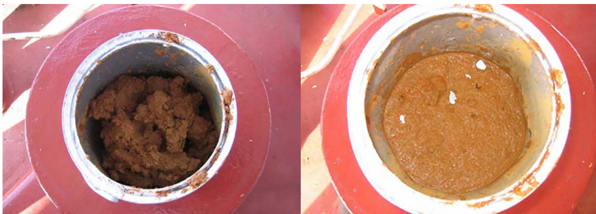
Figure 6 - Can test. The picture on the right shows formation of moisture at the surface, indicating that the moisture content may be too high and that more tests are needed to clarify the true relationship between MC and TML for that consignment.
