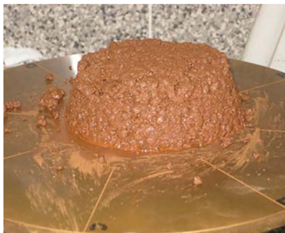
Figure 5 - Flow table test (Photo: Gard)
