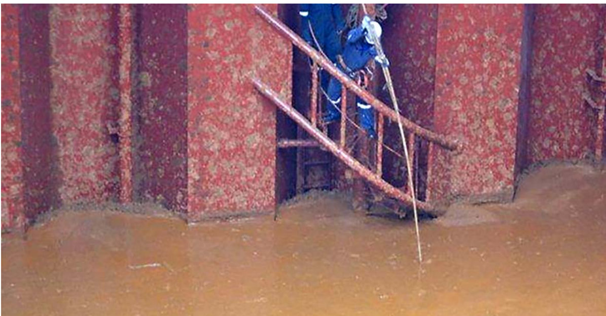
Figure 9 - Nickel ore liquefaction on a bulk carrier
