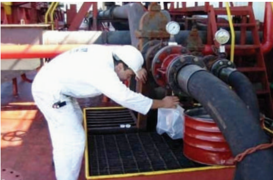
Sampling at ship manifold using DNV Petroleum Services Line sampler and cubitainer
